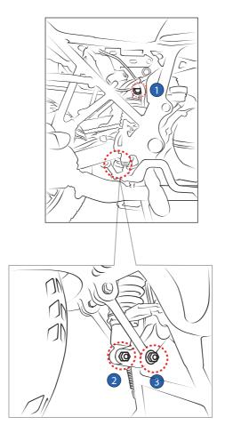
8 Install the hydraulic preload adjuster into the bracket by following the diagram below.
