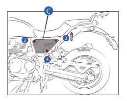
4 Remove the rear mudguard ® by loosening the screws ①② and ③④
