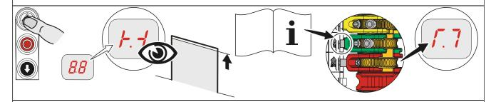
3. Move to CLOSE final limit position 5cm above the ground and adjust S5 pre-limit switch
