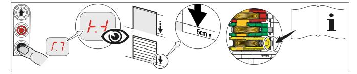
4. Move to CLOSE final limit position and adjust S4 CLOSE limit switch
