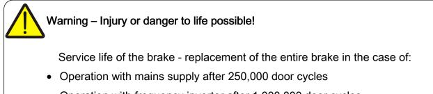
• Operation with frequency inverter after 1,000,000 door cycles
