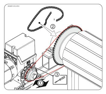
➤ Tighten the chain wheel properly (①/②).
