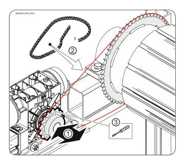
Tighten the chain wheel properly (①).
