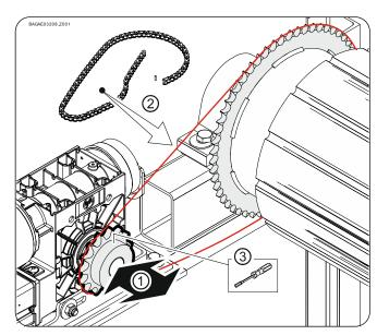
➤ Tighten the chain wheel properly (①).
