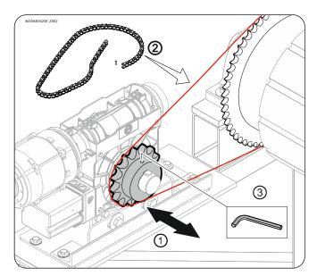
➤ Tighten the chain wheel properly (①).
