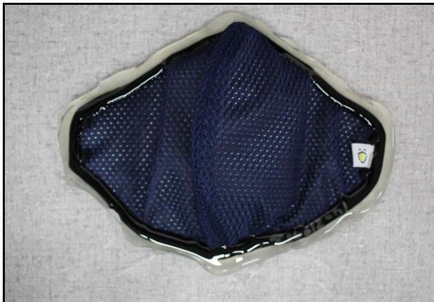
Figure 2: Typical sample affixed to test plate
