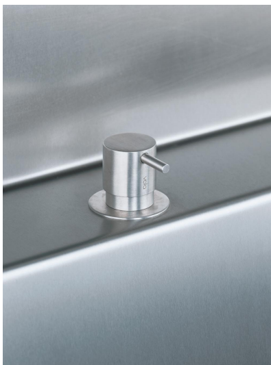
S50 Stop valve with 1/4 turn ceramic disc technology. Includes non-return valve and 1/2 inch inlet/outlet. Hole cut out size: 30 mm.
