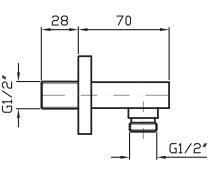
Wall elbow with round cover plate and 1/2" male water inlet connection. Crafted from solid brass.
