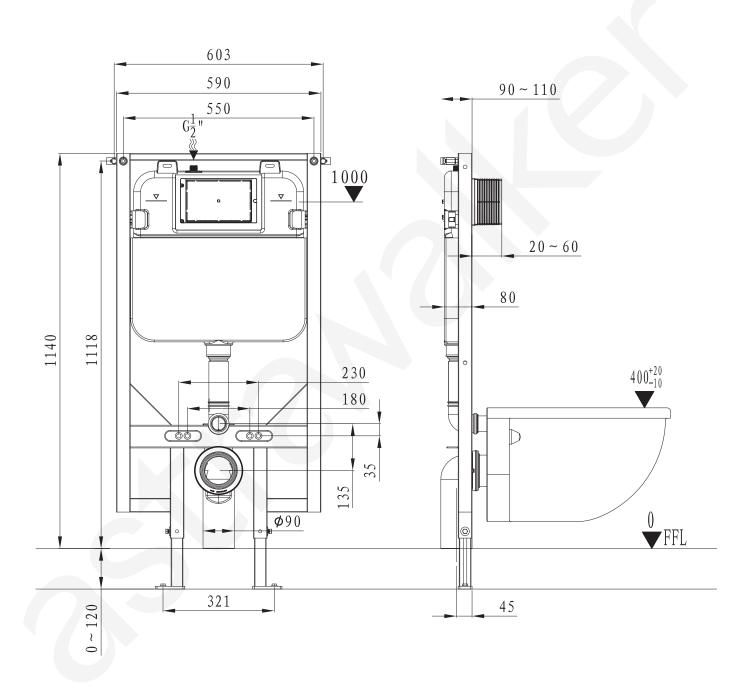
**NOTE**: There should be no gap between the wall & cistern frame. The wall should be made of noncompressible materials
