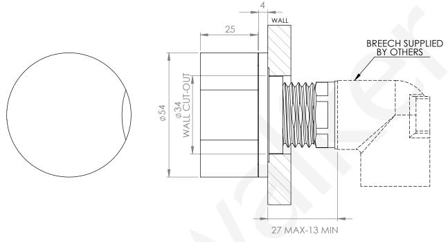
IMPORTANT: Front face of inwall body to finished wall face must be minimum 13mm to maximum 27mm
