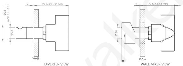
When installing the mixer ensure that it is positioned the correct way (as per markings on the body) with hot water on the left and cold water on the right when viewed from an operating position.
