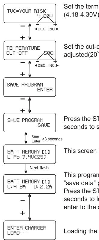
Set the terminal voltage, it can be adjusted (4.18-4.30V)
