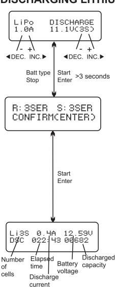
The value of discharge current on the left can not exceed 1C, and the value on the right can not be under the voltage recommended by the manufacturer to avoid over discharging. press the START/ENTER button for more than 3 seconds to start discharging.
