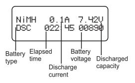
The screen indicates the discharging state. you can press START/ENTER button to alter discharge current, Press START/ENTER button again to store the value, Press BATT TYPE/STOP button to stop discharging. The emitted sound alerts the end of discharging.
