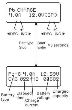
Set up the charge current on the left and nominal voltage on the right. Range of current 0.1-10.0A the voltage should match the battery being charged.
