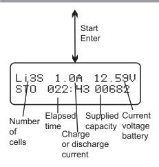
This screen shows the real-time status charging. Press BATT TYPE/STOP button once to stop the charge process.
