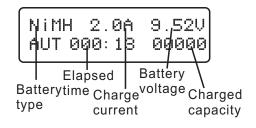
The screen displays real-time charging status. Press BATT TYPE/STOP button to stop the process.
