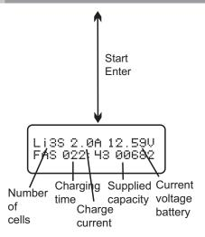
If both numbers are identical you can start charging process. If not, press BATT TYPE/STOP button to go back to previous screen to recheck the number of cells of the battery pack before going ahead.
