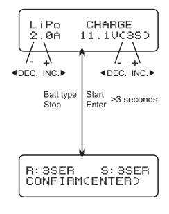
The left side of the first line shows the type of battery you choose. The value on the left of the second line of the charger is current the user sets. After setting the current and voltage, press the START/ENTER button for more than 3 seconds to start the process.
