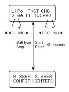
The value on the left side of the second lines shows the charge current. The value on the right side of the second lines shows the battery pack's voltage. After setting current and voltage, press the START/ENTER button for more than 3 seconds to start the process.
