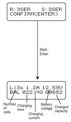
This screen displays the number of cells you set up and the processor detects.
