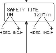
When you start a charge process, the integral safety time automatically starts running at the same time. This is programmed to prevent overcharge the battery if it proves to be faulty, or if the termination circuit cannot detect the battery full. The value for the safety time should be generous enough to allow a full charge of the battery.
