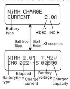
This program is for charging and discharging of NiMH/NiCD batteries associated with R/C models applications. You can press Inc. or Dec. button to change the parameter value, press START/ENTER button to store the value.
