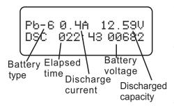
The screen display the real-time discharging status. Press START/ENTER button to change the discharging value. Press START/ ENTER button again to store the parameter value you set. Press BATT TYPE/STOP button to end the program.
