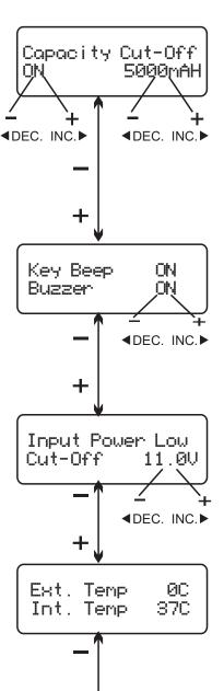
This program sets the maximum charge capacity that will be supplied to the battery during charge. If the deltapack voltage is not detected nor the safety time expired by any reason, this feature will automatically stop the process at the selected capacity value.
