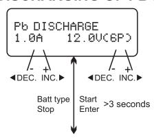
Set up the discharge current on the left and nominal voltage on the right. Range of discharge current is 0.1-5.0A the voltage should match the battery being discharged. Press ENTER/START button for more than 3 seconds to start discharging.
