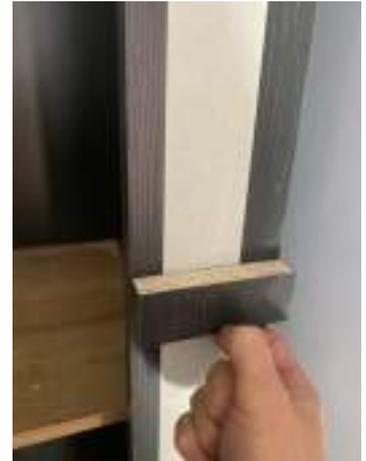
We are going to be using this block to draw the perfect image of our, wall, floor or ceiling directly on to our material, Because of the unique design and Fixing of the reference point of the “U-Scribejig” we have both hands free
