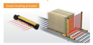
The muting actuator detects the surface of a passing workpiece. Even if a workpiece moves due to vibration, muting is kept enabled until the workpiece has passed. This prevents unexpected machine stops.
