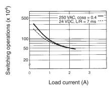
Reference: A maximum current of 0.6 A can be switched at  $125 \, \text{VDC}$  ( $\cos \phi = 1$ ). Maximum current of 0.2 A can be switched if L/R is 7 ms. In both cases, a life of 100,000 operations can be expected.
