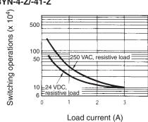
Reference: A maximum current of 0.5 A can be switched at 125 VDC ( $\cos \phi = 1$ ). Maximum current of 0.2 A can be switched if L/R is 7 ms. In both cases, a life of 100,000 operations can be expected.
