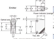
4-dia. vinyl-insulated round cable with 2 conductors (Conductor cross section: 0.2 mm² (AWG24), Insulator diameter: 1.1 mm), Standard length: 2 m
