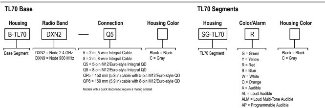
Select the 5-pin base for tower light configurations of up to three modules. Select the 8-pin base for tower light configurations of up to six modules, or when the event counter will be enabled.
