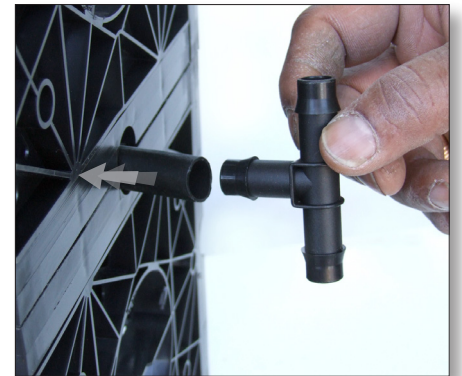
Insert the Tee-Connector at the other end.
