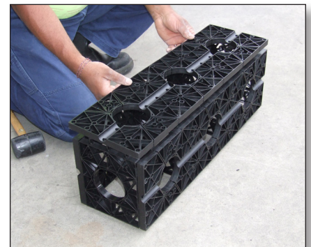
Turn module over and attach back plate. Ensure CHANNEL faces out.
