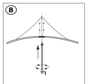
hold the cupola wrench to the bottom part of the cupola shaft and turn the wrench to raise the cupola until fabric becomes wrinkle free. Caution: do not over tighten!!
