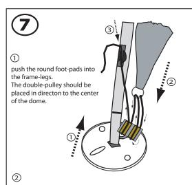
pull down the fabric (on the metal ring) and thread the corner ropes through the either left or right part of the pulley - after that thread the rope upwards through the metal ring and then again downwards through the second side of the pulley. Finally pull at the rope and tighten the dome "step by step" at all legs. Then thread rope into the plastic-cleat ③ at the frame leg. Please ensure that all legs are tensioned equally throughout the Dome.
