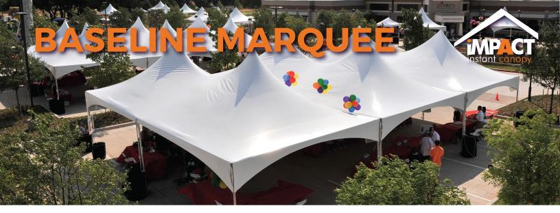
Our Baseline Marquee is constructed with heavy duty 2.5" aluminum tubing with extended sleeveson the footpads for extra reinforcement. The frame uses a tension wire system to support the roof and increase the strength and stability of the canopy. The top is made of Fire Retardant PVC Vinylwhich can be digitally printed with full color graphics. Also available in 10 different stock colors forunprinted shelters.
