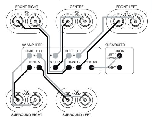
When running loudspeaker cables be especially careful not to run them across open floor areas where they could be a source of danger. Run loudspeaker cables around room boundaries whenever possible. Line level signal cables should be run away from mains cables. Never run line level signal cables parallel to power cables especially on long runs.
