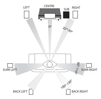
Above is the Dolby Labs recommended layout for 7.1systems. The 6.1 layout is the same except a single central speaker replaces the two back units. The 5.1 layout has no back speakers
