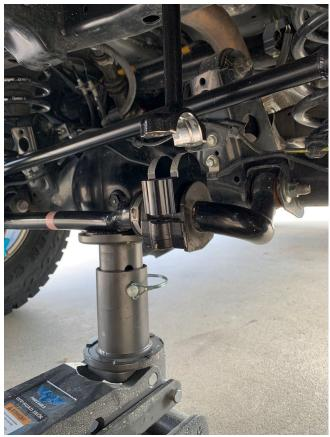
3. Jack the sway bar up so the end link is back together. Place the new, longer bolts and lock washers where the originals were and begin threading them in (your original bolts will no longer work, do not attempt to reuse them as they will not have the right length to hold the end links together). Alternating between them, tighten the bolts to factory spec (60ft/lb).
