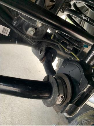
5. Once all 4 of those bolts are removed, lower the jack the same way you did on the passenger side, slowly until you can put the spacer in on the driver's side with it still supporting the sway bar (again applying the recommended anti-seize on top of the spacer).
