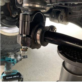
7. Once the bolts connecting the spacer are tight, lower the jack and reposition it to under the arm that connects the sway bar to the axle on the driver's side (should be the only thing left to reconnect). Use the jack to help you re-align the arm with the axle connection by raising it up.
