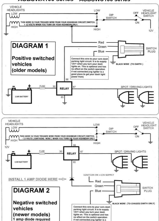
If you are using this switch for a compressor, fridge or non-lighting accessory follow diagram 1 and use a fused 12 volt supply in place of the lighting circuit.
