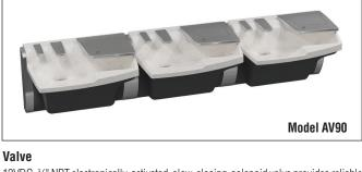
12VDC, %" NPT electronically-activated, slow-closing solenoid valve provides reliable performance since there are few moving parts, and its operation is unaffected by most chemicals and minerals often present in municipal water supplies. Operating water pressure range is 20-80 psi. Flow regulator keeps flow rate constant at all pressures.
