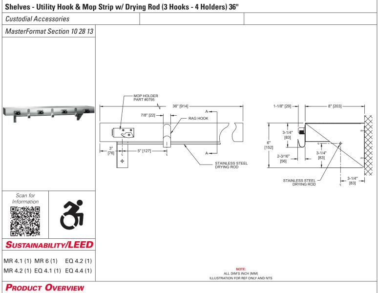
Shelf fabricated of 18 gauge type 304 satin finish stainless steel, this shelf is 8" [203] deep with 3/4" [19] return for rigidity, mounting brackets shall be 16 gauge same material. Mop holders are riveted to strip, and rubber cam is ribbed for grasping. Rod and hooks for wet rags are included. 4 mop holders/3 rag hooks, 36" [914]. Pivoting spring loaded holders have serrated rubber cams for grasping.
