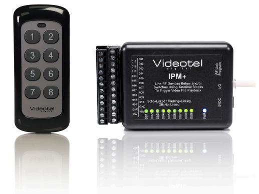
The serial data sent to the player is the file number the player is to play. The format of the serial data being sent is TTL voltage levels of 0 volts to +5 volts. It is transmitted at 4800 Baud and a data length of 8 bits. It has no parity bit and 1 stop bit.
