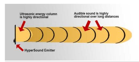
HyperSound generates an ultrasonic energy beam that is highly directional, and converts to audible sound in the air. The length of the column determines the directionality at audio frequencies. This sound is directional over longer distances than traditional loudspeakers.
