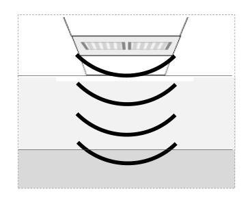
The parametric loudspeaker provides an effective means of projecting sound in a highly directional manner, without using large loudspeaker arrays, to form sharp directional beams.<sup>6</sup>
