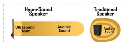
HyperSound travels in a focused direction along the beam, unlike typical point source loudspeakers that emit sound waves in all directions.
