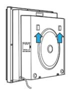
7. Once the bracket has been properly affixed to the wall, align the bracket pockets with the hooks and slowly slide the unit down onto the bracket's hooks.
