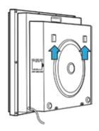
7. Once the bracket has been properly affixed to the wall, align the bracket pockets with the hooks and slowly slide the unit down onto the bracket's hooks.
