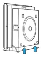
1. Remove the screws that secure the base stand to the unit.
