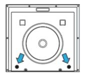
6. Place the two included adhesive discs onto the small circles on the back of the unit.
