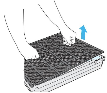
4. Remove the white Medium Filter from the black frame to discard the plastic wrapping. Return the filter to its frame.
