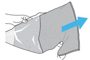
7. Pull out the Activated Carbon Filter and discard plastic wrapping.
