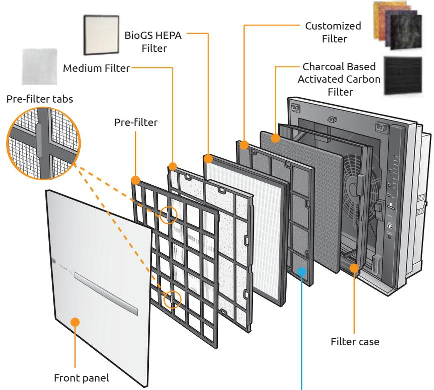
9. Return filter case to the unit. Slide the bottom of the case back into the unit (1), then press the top in (2).
