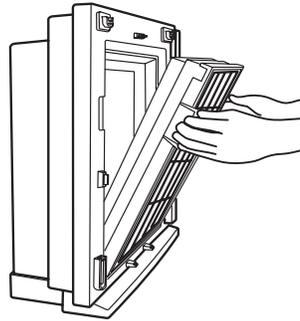
3. Pull the tabs on the front of the Pre-filter to remove it.
