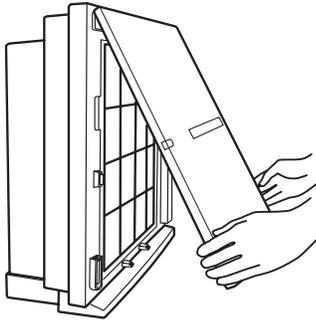
2. Remove the filter case by grasping the handles on either side and pulling forward. Lay the filter case on a flat surface.
