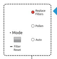
5. Once you have replaced the filters, press and hold the Mode/Filter Reset button for three seconds, or until the Replace Filters Indicator clears itself.
