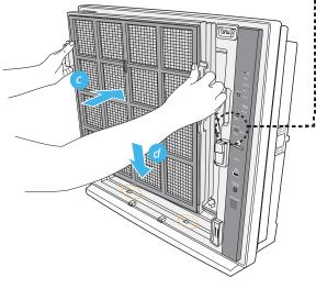
4. Return filter case to the unit. Slide the bottom of the case back into the unit (c), then press the top in (d).
