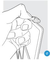
First, remove the Pre-Filter by pinching the two tabs on top, and lifting out (a).
