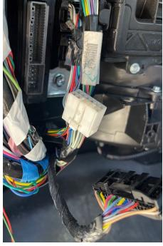
Step 6: Install the 40 pin and 10 pin jumper Harnesses into the 4x4 module and connect to the main wiring harness as shown in pictures
