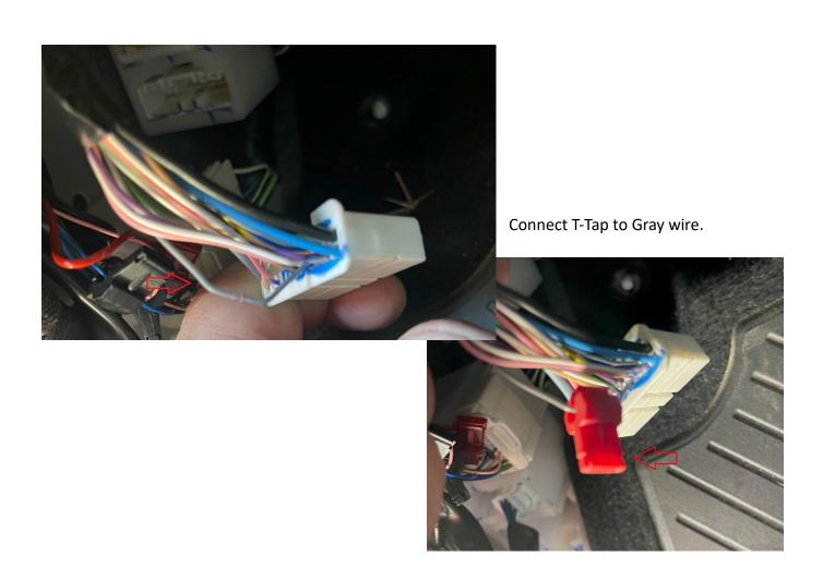
Step 11: Connect the AnyTime Locker's Gray/white wire with provided spade connector to the T-Tap and tie up and loose wires.
