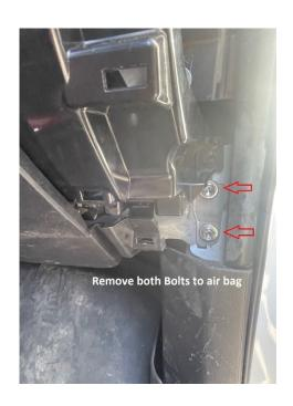
Step 4: Remove all screws holding in the glove box,
