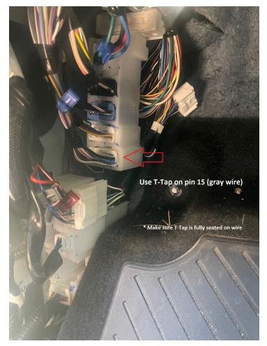
Step 10: connect the T-Tap to the Gary wire on connector IA5.
