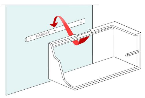
5. While two people hold the vanity base in place, the third person marks screw placement in the top rail in the back of the vanity, making sure they are in line with the screws in the hanger and aligned with the studs. Then drill guide holes and secure vanity to the wall with lag screws and washers.
