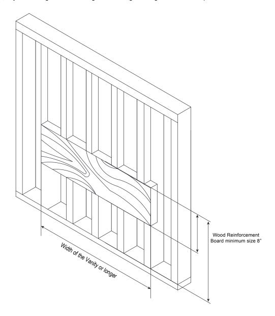
STEP 1. Cabinet positioning and installation
