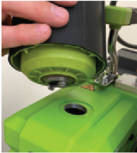
FIGURE 7: Demister removed, showing oil opening
