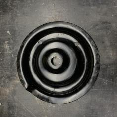
Push the smaller diameter recess integrated into the adapter mount into the stock cup on the spring perch until it seats firmly, flat, and without movement.
