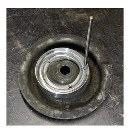
10. Remove the 6mm bolt, and the adapter then repeat step 6 for the other three indentations.
