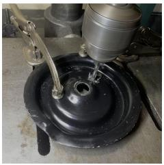
Make sure to remove any burrs created on both sides of the perch by using a file, deburring tool, or sand paper. (Optional, Drill with appropriate size countersink)
