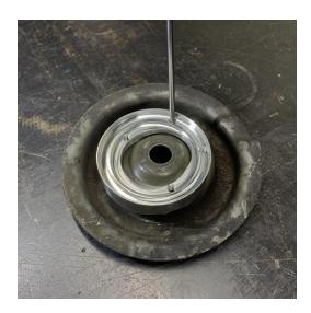
4. While holding the mount position, use a hammer to strike the center punch and create a recess.
