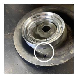
3. Align the supplied center punch into one of the four holes
