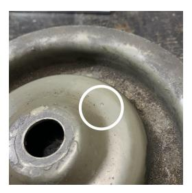
6. Use the supplied drill bit to create a hole centered on the indentation created with the center punch.
