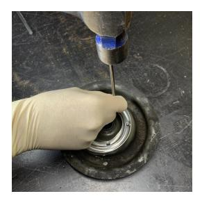
5. Remove the mount from the perch (recess is shown below)
