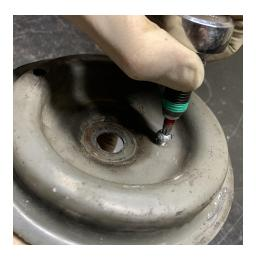
9. Use the supplied center punch once again to create indentations using the other three holes. (Ensure that the adapter does not move when using the center punch and it stays flat against the stock perch surface.)
