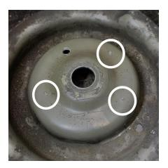
11. Bolt the adapter to the newly created and deburred holes.
