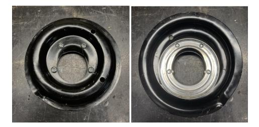
12. Using a die grinder, file, or hole saw to enlarge the center opening you can use the 240 Top Mount as a guide. Enlarge the opening until you are able to see the lines pointed at below.
