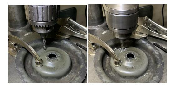
Make sure to remove any burrs created on the perch's back and front side by using a file, deburring tool, or sandpaper. (Optional, Drill with appropriate size countersink)
