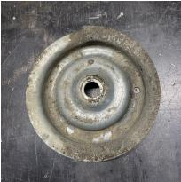
1. Push the smaller diameter recess integrated into the mount into the stock cup on the spring perch until it seats. (Ensure that the adapter is flat and not raised on the fillet)
