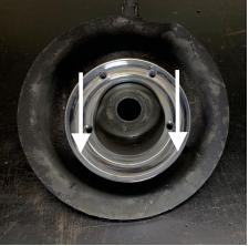
2. Clock the mount so that the blunt line (pictured below) is aligned with the singular drain hole (Ensure that the mount is flat and not raised on the fillet)
