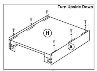
Take Drawer Bottom (H) & turn it over onto it's face. Use (6) Small Screws to attach the Metal Box Sides (A) to the Drawer Bottom. Shown above.
