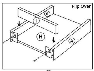
Slide Drawer Back (1) into 90 degree angle against the Metal Box Sides (Shown above) and use (2) Small Screws to secure into place.
