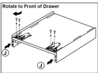
Attach Drawer Glide Release Clips © & screw them into place as shown. Use the mechanism to dislodge the Mounting Brackets J in order to attach them to the Drawer Face (X).
