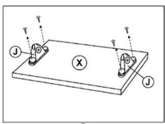
Take Drawer Face (X) (included in a separate package) & use (4) Small Screws to secure Mounting Brackets (located inside Metal Box Sides). Method Shown above.
