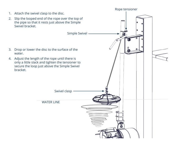
When the AquatiClear is operating, the disc will be pulled toward the whirlpool to float just above it.
