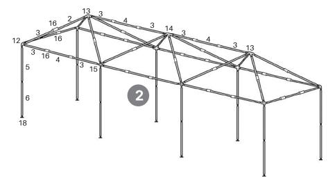
Step 3 Assemble the roof cover and finish the mainframe.
