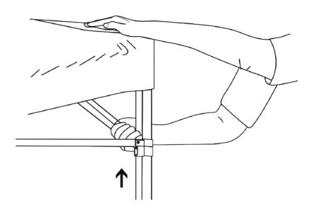
Step 4 Extend the legs and adjust them to a proper height by pressing down the leg-release buttons.
