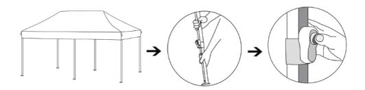
Step 5 Attach the sidewalls to the frame with built-in Velcro tapes as per your needs.
