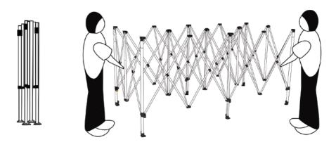
Step 2 Attach the roof cover to the frame by matching the hook and loop straps inside the 4 corners of the roof cover with the hook and loop straps at each frame corner, then fully unfold the frame.
