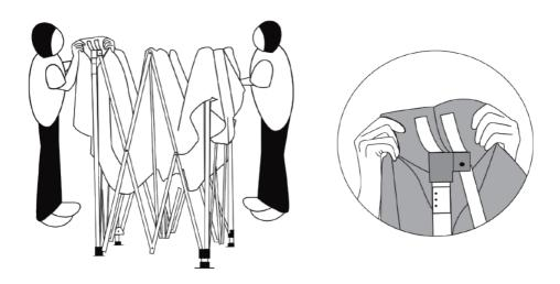
Step 3 Attach the roof cover to the frame by matching the hook and loop straps inside the 4 corners of the roof cover with the hook and loop straps at each frame corner, then fully unfold the frame.
