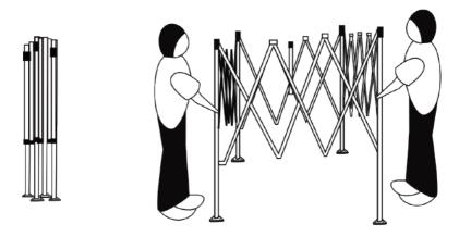
Step 2 Attach the roof cover to the frame by matching the hook and loop straps inside the 4 corners of the roof cover with the hook and loop straps at each frame corner, then fully unfold the frame.
