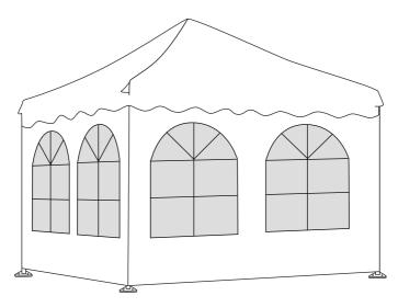
Step 6 Secure the whole structure with the anchoring accessories. You can also use some extra weights (for example, sandbags) to weigh down your canopy.
