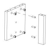
3 Place the shelf on the front panel and tighten the screws
