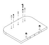
7 Place the table top and shelf on the back panel and tighten the rest of the screws.
