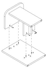
Join the table top and the front panel and tighten the screws
