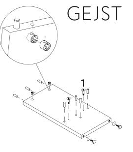
2 Insert the housings and dowels in the bottom of the shelf and connect the beam
