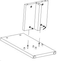
4 Insert dowels, housings and bolts on the table top
