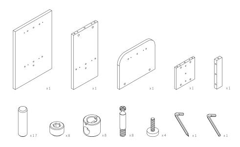
Start by attaching the dowels, house, bolts and feet to the front panel
