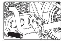
Open the charging port cover, plug in and charge.
