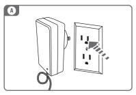
Plug the charger plug into the wall outlet. The light on the charger should be green. Note: Try a different outlet if the green light (LED) does not turn on.
