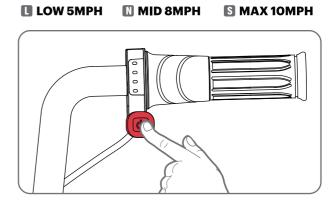
**Gear switching -** The default speed gear is toddler mode (L) when starting up. Short press it the power button once to switch to N, and short press again to switch to S. Repeat this proces to cycle through the gears. When switching gears, the battery indicator light will also flash.
