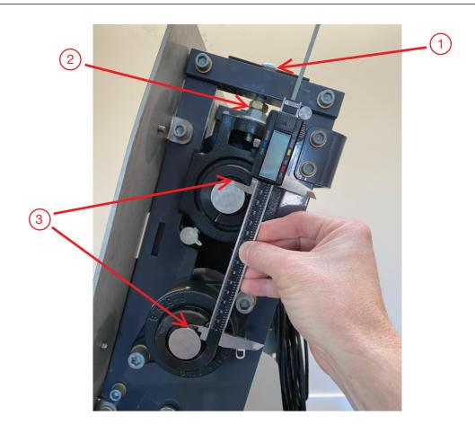
Factory roller tension settings are critical to a properly functioning machine. Perform the following steps to return your machine to factory settings.
