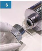
Hand-screw closed end nut on the reactor chamber closed end of quartztube) to protect the o-ring, do not over tighten.
