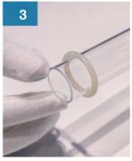
Install o-ring onto the open end of quartz tube (~0.5inch from the edge).
