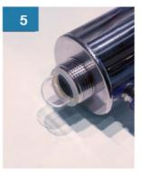
Install o-ring onto the closed end of quartz tube.
