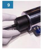
Install the cover cap and hand-tighten onto open end nut .
