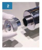
Remove the open end nut from reactor chamber open end.
