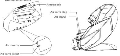
▶ Hold the armrest unit up and hook the bracket 2 onto the carrier groove, slowly push the armrest unit back into the chair linkage until bracket 2 aligns completely with bracket 4, insert bracket 1 into bracket 3, use a screw to secure the armrest into place. (Same installation method with the other side)
