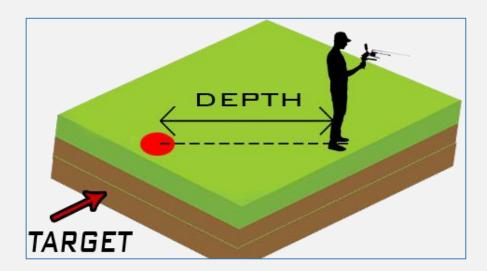
Measure the distance between the antennas reversing back and the target center point.
